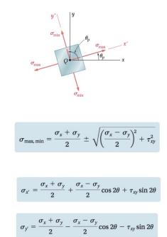
$$\sigma_{\max,\min} = \frac{\sigma_x + \sigma_y}{2} \pm \sqrt{\left(\frac{\sigma_x - \sigma_y}{2}\right)^2 + \tau_{xy}^2}$$
